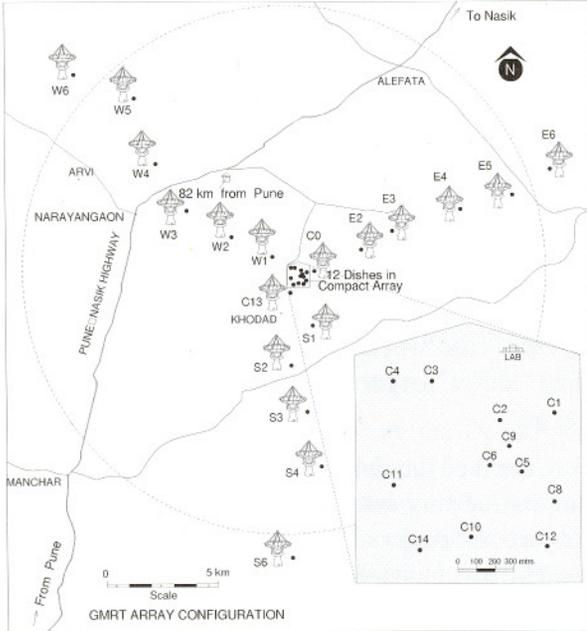
**Fig. 1:** Layout of the antennas of GMRT. The central square is shown in the inset.
