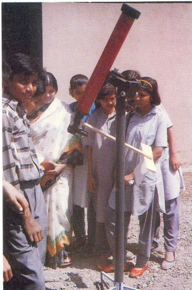
This photograph shows the projection screen mounted on a 3 inch CSIO telescope.
