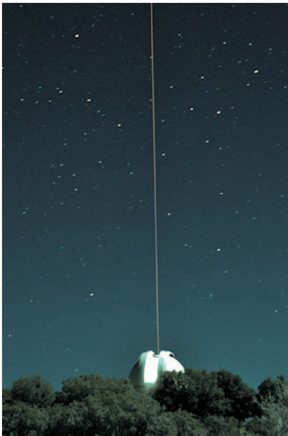
Figure 31: A false colour image of the first propagation of the Robo-AO laser guide star from the Palomar 60 inch telescope
