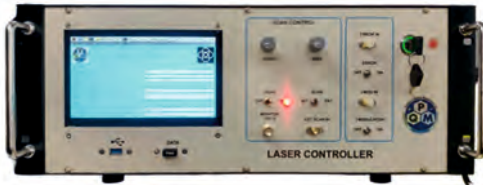
Figure 17: Complete extended cavity diode laser (ECDL) controller.
