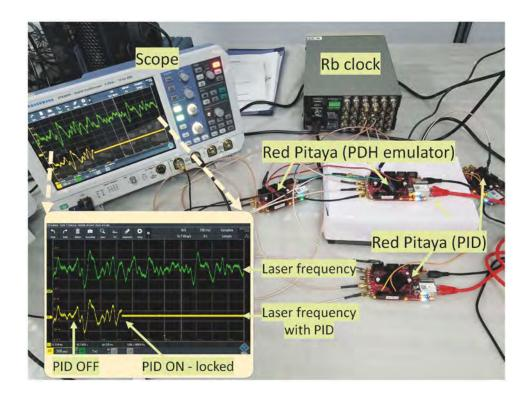
Figure 27: Experiment setup demonstrating the emulated locking of a laser to an ultra-stable cavity using an FPGA-based PID controller. Note the steady/locked laser frequency when the PID is turned on, in the inset.
