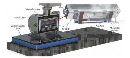
Figure 25: Fabry-ProtCavity is housed in an ultra-high vacuum chamber and three layers of thermal shields. The entire assembly is placed on an active vibration isolation table.
