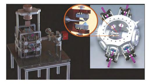
Figure 24: The design of the science chamber that consists of the ultra-high vacuum container, magnetic coils along all three directions, helical resonator, and high-resolution imaging system.
