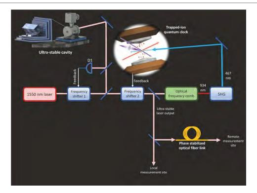
Figure 23: Schematic of the experimental setup that consists of three major sophisticated technologies: ytterbium-ion-based optical clock, generation of sub-Hz linewidth & ultrastable laser, and phase stabilization of optical fiber.
