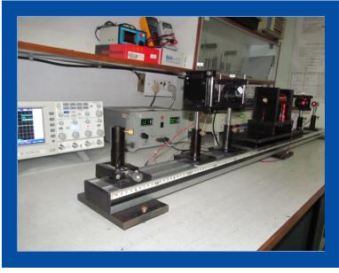
The laser will act as a carrier and the audio is given as a modulating signal to the solenoid, the audio signal modulated in the presence of Faraday material (TGG) and demodulated by converting polarization modulation into intensity modulation at the photo detector. The power requirement is very low as compared to the existing analog modulation techniques. The system is successfully working over the audio bandwidth.
