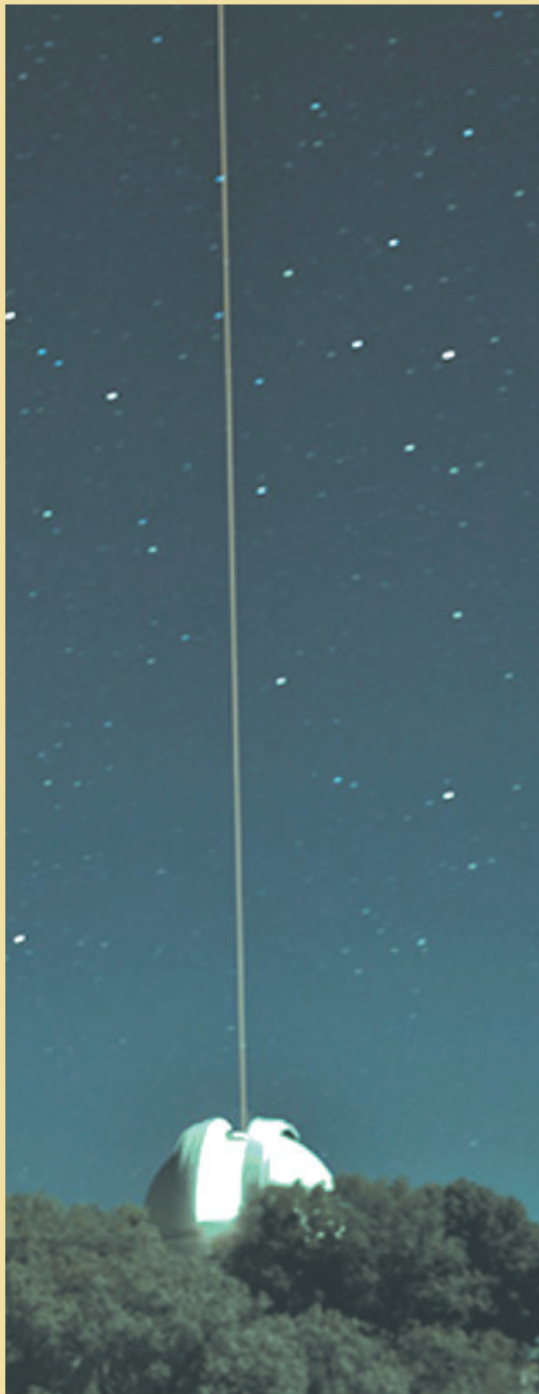
Laser beacon guide star being test fired from the Palomar 60 inch telescope during an engineering run in September 2010.
