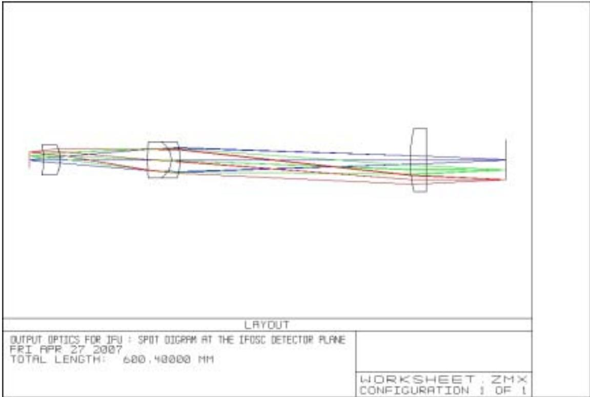
Figure 19: Optical layout of the Output Optics
