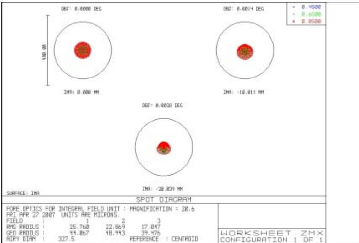
Figure 18: Performance of the Fore Optics: Spot Diagram; For the magnification of 20.6
