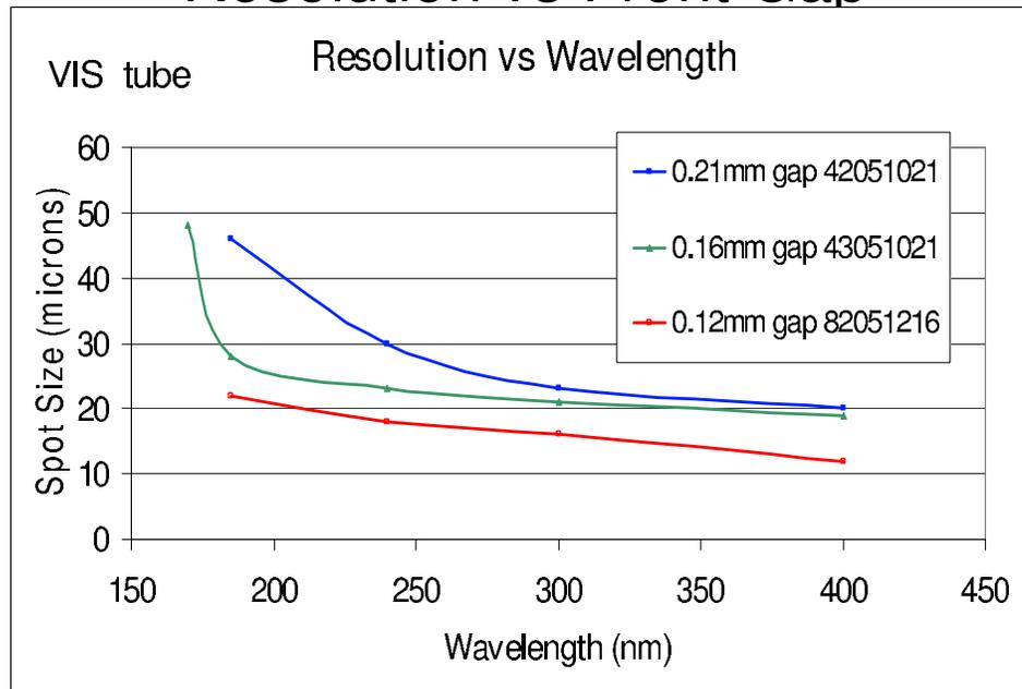
Figure 21: The dependence of spatial resolution of a detector is shown, for three values of the gap between photo-cathode and MCPs, as a function of wavelength, (from a report by Photek Ltd. UK)
