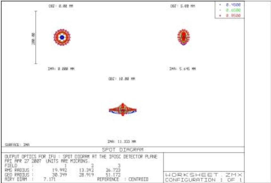
Figure 20: Performance of the Output-optics: Spot diagram at the IFOSC detector plane
