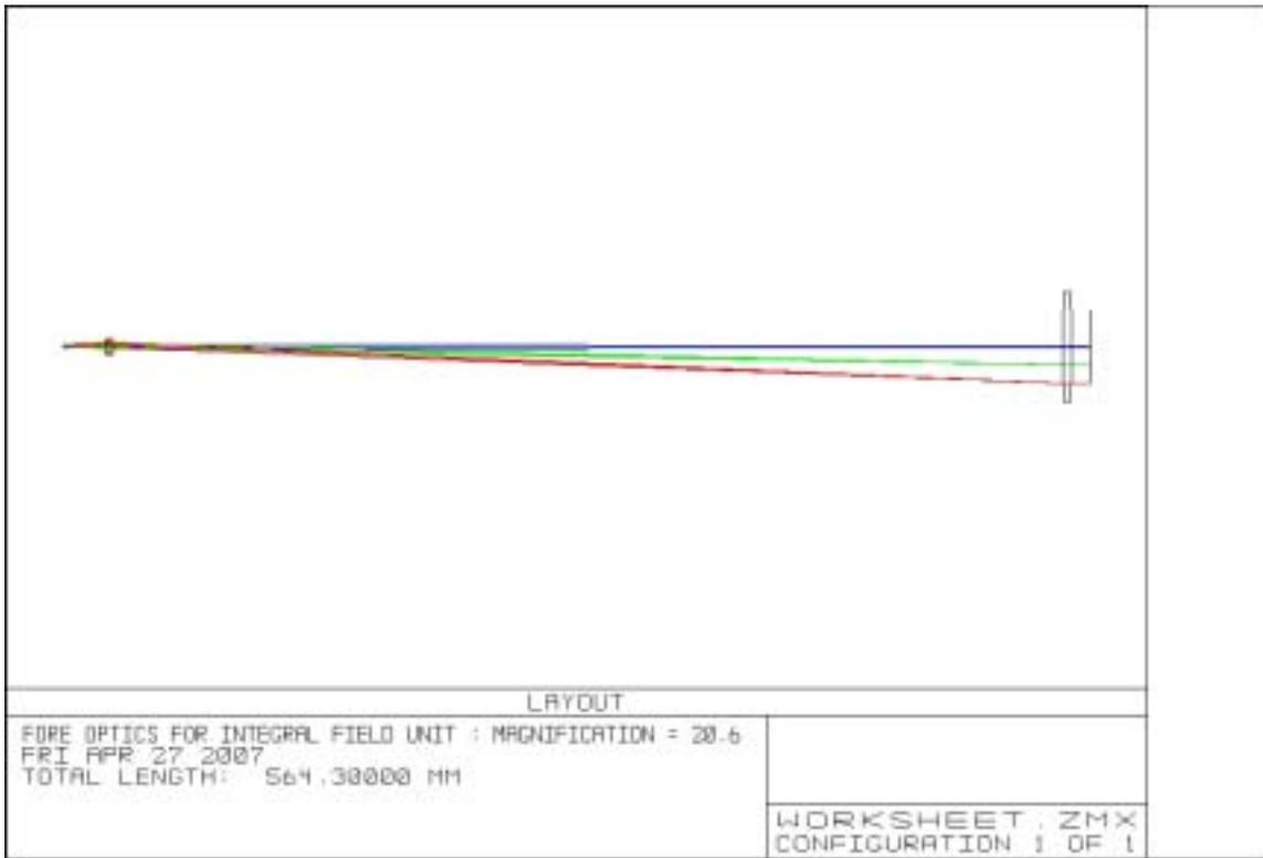
Figure 17: Optical layout of the Fore-Optics for the magnification of 20.6
