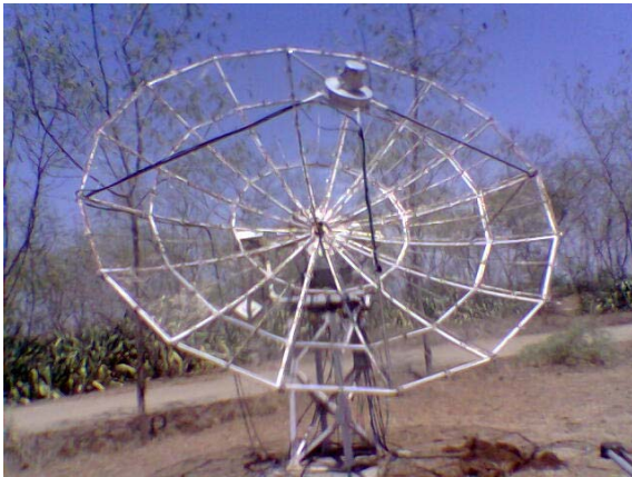
Figure 18: Top Panel: Two high efficiency feed systems fabricated by engineering students for 21cm (1420 MHz) radio astronomy observations. Left: A ‘Chaparral’ type feed horn containing multiple choke-rings or low-Q traps for higher gain and bandwidth. Right: A cavity backed dipole feed showing wide usable bandwidth range of 1.3 GHz. Lower Left Panel: The 21cm feed-horn is shown mounted at the focus of 4-m diameter radio antenna located at the GMRT observatory. Lower Right Panel: Raw data received with the 4-m radio dish antenna. It shows a complex 21cm hydrogen line spectrum from the direction of galactic Perseus and local arms. The x-axis shows Doppler shifted frequency in KHz, with red section denoting red-shift (+ve velocity) and the blue section denoting the blue-shift (-ve velocity). The y-axis is proportional to radio power or antenna temperature
